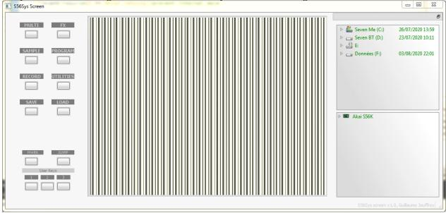
You have probably loaded the software before your computer recognized the sampler. Please restart the software without turning off the sampler. If this does not work you may have driver issues, please contact support at <u>s56sys@free.fr</u>.
